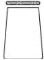
4 Saldobrasatura bordo Braze-welding
