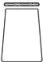
4 Saldobrasatura bordo Braze-welding
